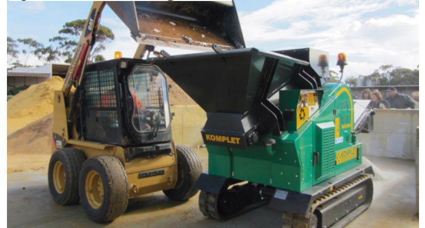
Figure 27 – Glass crushing machine
